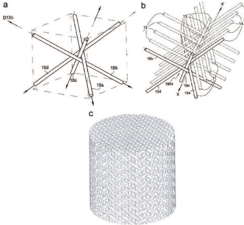
Fig. 5. (a) Tubes fitting according to the four diagonals of a cube, (b) reproduction of the layout in one direction, and (c) final structure.
