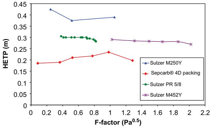
Fig. 18. Comparison of the HETP of the Sepcarb<sup>®</sup> 4D packing and standard packings.
