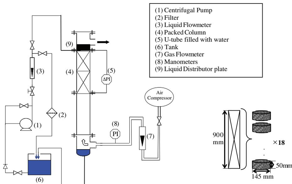
**Fig. 8.** Experimental setup for hydraulics experiments.
