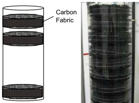
**Fig. 13.** Packing setup of 1st series of runs.
