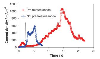
**Fig. 4** Effect of anode pre-treatment on current generation. Chrono-amperograms on graphite felt pre-treated by yogurt waste adsorption (*open square*) and control electrode not pre-treated (*open triangle*). Polarization at +0.1 V versus SCE in compost leachate. Arrow indicates yogurt-waste substrate addition
