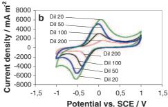
electrochemical cells and refilling with dilutions (20–200 times) of yogurt waste. **b** Cyclic voltammetry carried out at end of chrono-amperometry, 13 and 20 days. Scan rate 10 mV s $^{-1}$
