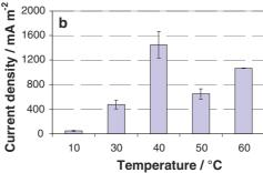
Example of chronoamperogram at  $60\,^{\circ}$ C. Arrow indicates substrate addition. **b** Maximal current density reached at different temperatures. Error bars correspond to 2–6 replicates
