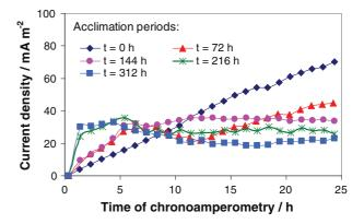
Fig. 2 Effect on current generation of acclimation of the inoculum to yogurt waste substrate. Chronoamperogram on graphite felt polarized at  $+0.1~\rm V$  versus SCE in compost leachate, which had been acclimated for increasing periods from 0 h to 312 h. The x-axis gives the time from beginning of chronoamperometry. The acclimation periods that preceded chronoamperometry are given as the label of each curve
