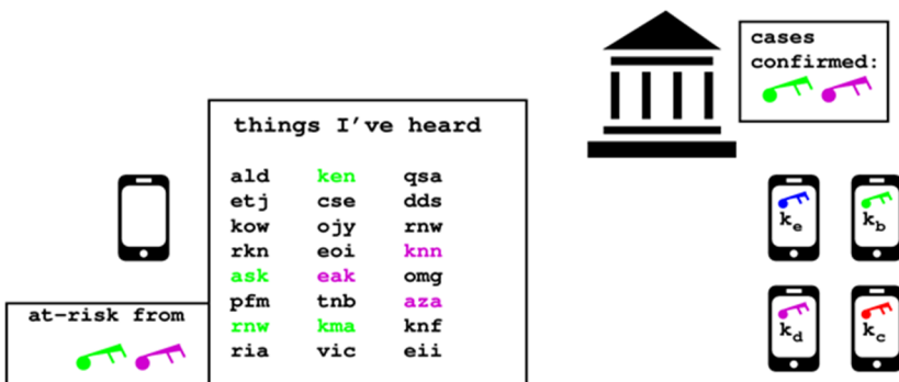
Figure 4. Decentralised model: the app retrieves encryption keys from app users who have tested positive and can use these to search in the contacts registered locally.
