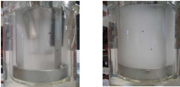
Fig. 4 Aspect of the reacting medium with ultrasound ( P = 16 and 67 \text{ W} )
