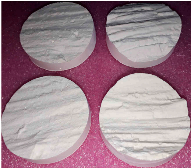
FIGURE 4 | Plaster faults made using the 3D-printed molds (i.e., an example of which is shown in Figure 3 ). (Left) S_m (top) and its complementary surface (bottom) . (Right) S_{mm} (top) and its complementary surface (bottom) . The samples have a diameter of 40 mm. One can appreciate that the fault at the millimeter scale ( S_{mm} ) shows a higher roughness aspect than at the meter scale ( S_m ).
