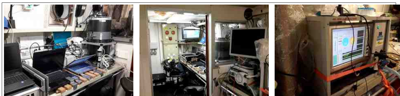
Picture of the Téthys II wet lab during the cruise with the sensors for the TSG+ sampling: Automated flow cytometer (left); pCO 2 (center); Pocket Ferry Box (right).
