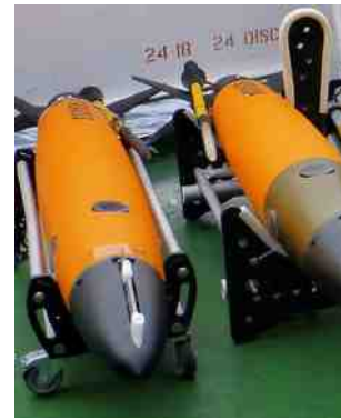
SeaExplorer gliders SEA003 and SEA004. One specific aspect of their design is the absence of side wings which make their deployment easier from smaller boat. This glider is also the only one manufactured in Europe (photo credit: Alseamar).
