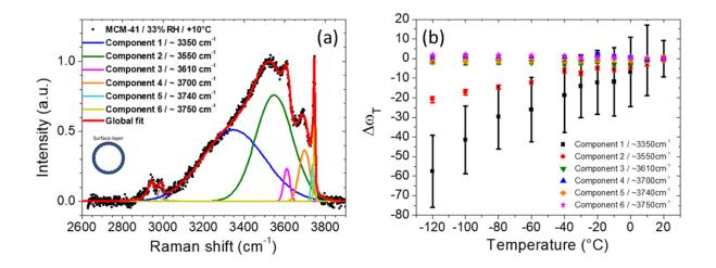
Figure 7. (a) Fit (thick red line) of a sum of Gaussian peaks (solid thin lines) to the experimental Raman spectra (solid circles) of partially filled MCM-41 at 33% RH corresponding to the formation of a surface water layer. (b) Temperature dependence of the frequency of the different bands.
