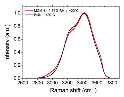
Figure 2. Raman spectra in the O-H stretching region of bulk water and water-filled MCM-41 recorded at 20  $^{\circ}$ C.
