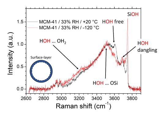
Figure 8. Comparison of the Raman spectra of partially filled MCM-41 at 33% RH acquired at the two extreme temperatures, -120°C (red line) and 20°C (black line).
