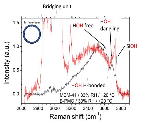
Figure 9. Comparison between the Raman spectra of a water layer adsorbed at 33% RH in B-PMO (red line) and MCM-41(black line) samples.
