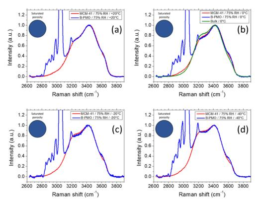
Figure 5. Raman spectra in the O-H stretching region of confined water in fully filled MCM-41 (red line) and B-PMO (blue line) recorded at (a) 20 °C, (b) 0 °C, (c) -20 °C and (d) -40 °C.
