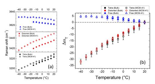
Figure 4. (a) Temperature dependence of the band positions obtained by the fitting procedure of the intramolecular O-H stretching in bulk water and confined water. (b) Temperature dependence of  $\Delta\omega_T = \omega_T(T) - \omega_T(T=20^{\circ}C)$ . Solid lines are guides to the eyes.
