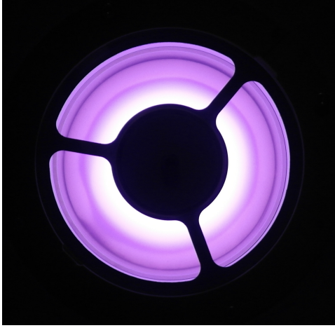
Fig. 6. Photograph of AIPE thruster operating with 10 sccm of Kr at 140 W. Grids have been removed.
