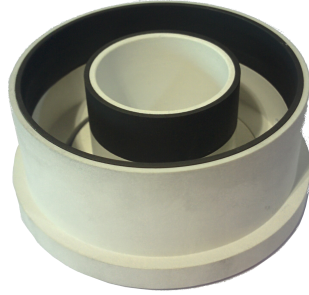
FIG. 3. Discharge channel with the graphite inserts. The graphite inserts cover two thirds of the discharge channel length.
