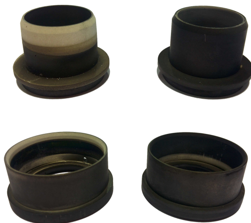
Figure 8. Ceramic walls of the ISCT200-US (left) and ISCT200-MS (right) highlighting, for the MS case, the absence of the characteristic erosion pattern in the black deposit formed on the walls.
