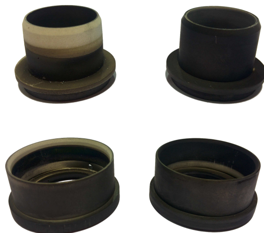
Figure 8. Ceramic walls of the ISCT200-US (left) and ISCT200-MS (right) highlighting, for the MS case, the absence of the characteristic erosion pattern in the black deposit formed on the walls.
