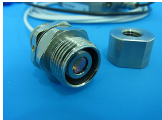
Fig. 5. Pyrometer sensor head with housing.
