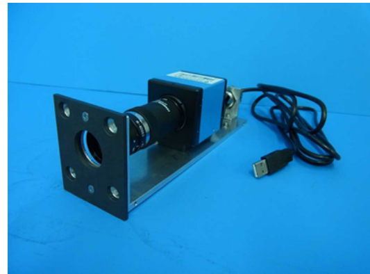
Fig. 4. Telemicroscope with housing (without metal cover).
