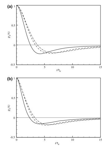
**Fig. 9.** Acceleration auto-correlation function. (a) Solid line, *B*1; dashed line, *N*1; dash dot line, *S*1. (b) Solid line, *B*2; dashed line, *N*2; dash dot line, *S*2.
