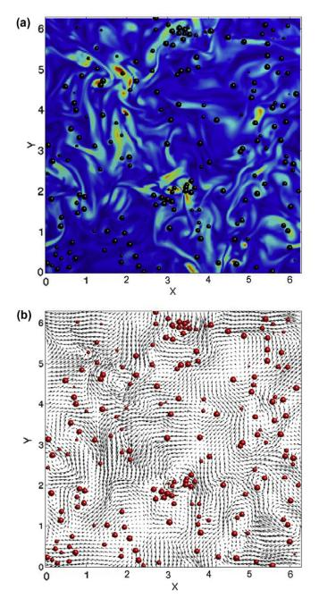
**Fig. 1.** (Color online) (a) Instantaneous bubble positions and enstrophy level (case *B*1). Bubbles are displayed with their actual size in the planar slice, with high enstrophy levels shown as white. (b) Corresponding view of bubble positions and fluid velocity, shown by the vector arrows.
