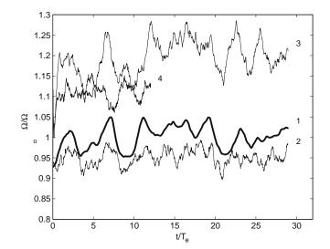
**Fig. 2.** Sample Lagrangian time-history of rms vorticity fluctuations following the bubbles or particles, corresponding to cases S1 and B1: (1) single phase flow; (2) particles (S1); (3) bubbles simulated with force monopole only (B1-M); and (4) bubbles (B1).
