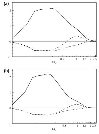
**Fig. 6.** Determination of the effective viscosity. (a) Solid line, dissipation rate spectra (*N*1); dashed line, dipole energy transfer (*N*1); dash dot line, corresponds to  $v_{add}/v = 0.150$ . (b) Solid line, dissipation rate spectra (*N*2); dashed line, dipole energy transfer (*N*2); dash dot line corresponds to  $v_{add}/v = 0.105$ .
