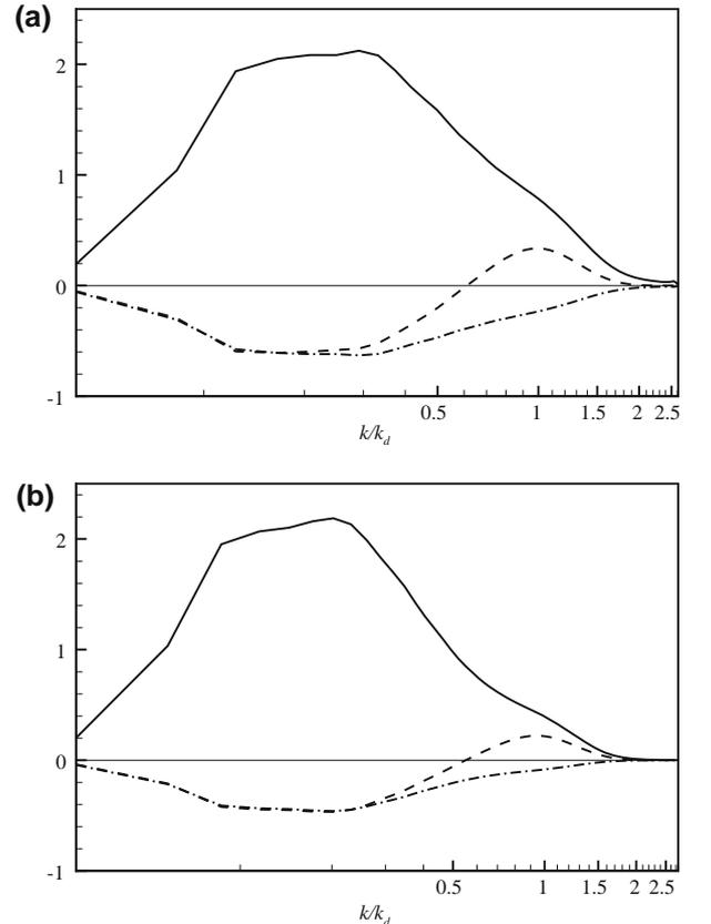
**Fig. 6.** Determination of the effective viscosity. (a) Solid line, dissipation rate spectra ( $N1$ ); dashed line, dipole energy transfer ( $N1$ ); dash dot line, corresponds to  $\nu_{add}/\nu = 0.150$ . (b) Solid line, dissipation rate spectra ( $N2$ ); dashed line, dipole energy transfer ( $N2$ ); dash dot line corresponds to  $\nu_{add}/\nu = 0.105$ .
