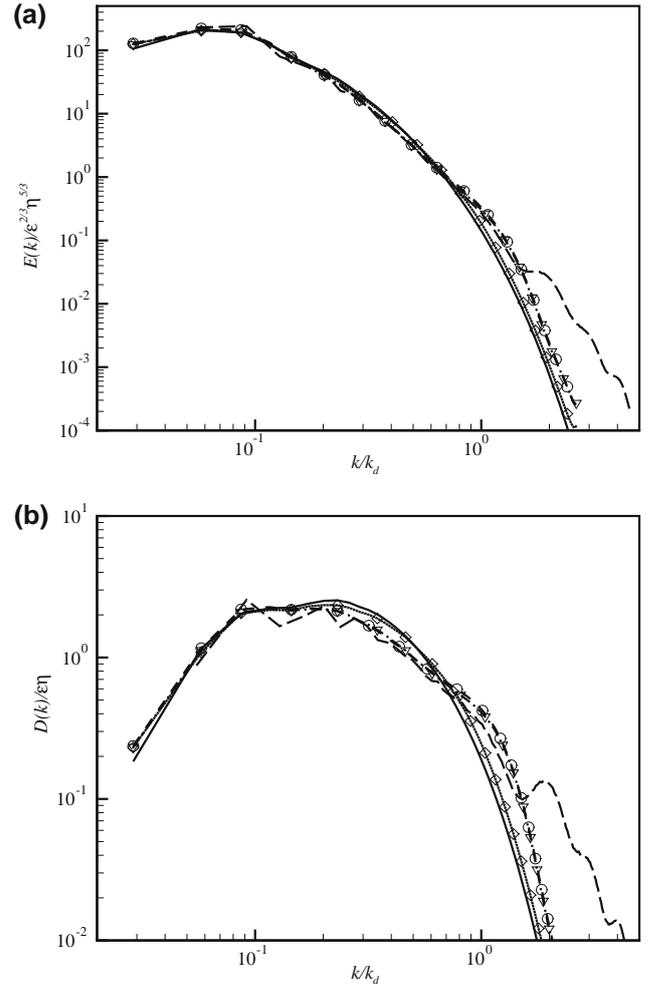
**Fig. 4.** Energy (a) and dissipation (b) spectra (grid  $192^3$ ). Solid line, single phase flow; dashed line with circles, bubbles B2; dash dot line with triangles, solid particles S2; dotted line with diamonds, solid particles S2-M; Long dash line, dataset S2 from (ten Cate et al., 2004).
