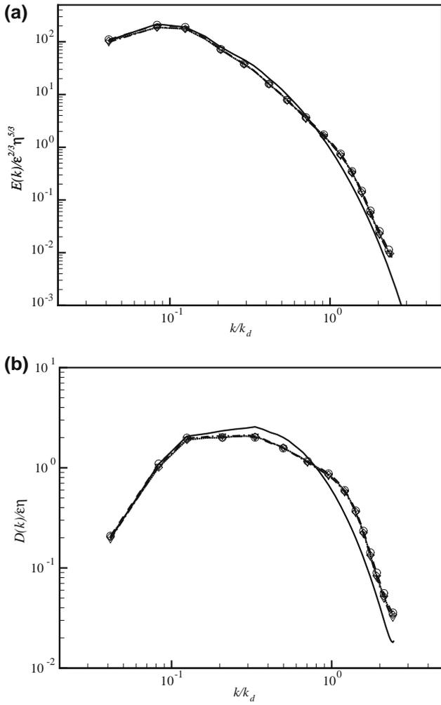
**Fig. 3.** Energy (a) and dissipation (b) spectra (grid  $128^3$ ). Solid line, single phase flow; dashed line with circles, bubbles B1; dash dot line with triangles, neutral particles N1; dotted line with diamonds, solid particles S1.
