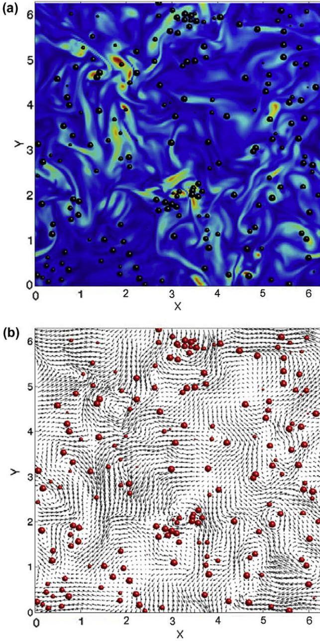
**Fig. 1.** (Color online) (a) Instantaneous bubble positions and enstrophy level (case B1). Bubbles are displayed with their actual size in the planar slice, with high enstrophy levels shown as white. (b) Corresponding view of bubble positions and fluid velocity, shown by the vector arrows.
