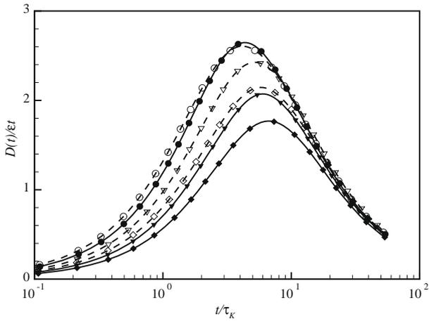
**Fig. 10.** Normalized velocity structure function. Solid line with solid circles, B1; solid line with solid triangles, N1; solid line with solid diamonds, S1; dashed line with open circles, B2; dashed line with open triangles, N2; dashed line with open diamonds, S2.
