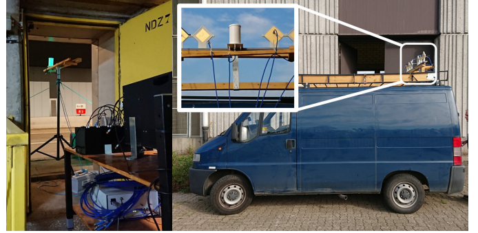
Fig. 2. Measurement campaign with the Tx in the tunnel and the Rx in the van
