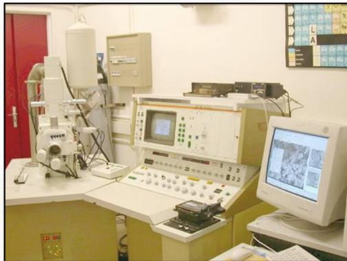
JEOL Scanning Electron Microscope - JEOL 840A
