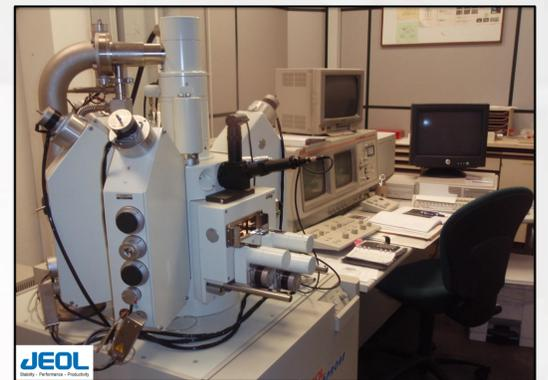
Electron Probe Micro-Analyser (EPMA - JEOL 8800) Equipment: 5 wavelength dispersive x-ray spectrometers (WDS) each with two crystals
