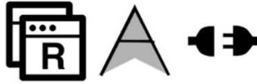
Fig. 4 Three possible strategies for embedding a shortcut cue in an icon. Left: the R is simply added on the icon. Center: the A leverages the shape of a pointer icon. Right: the E letter leverages the negative space of the power socket icon
