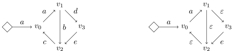
(a) Original control-flow graph for two cache sets: \{a, e\} and \{b, c, d\} .
