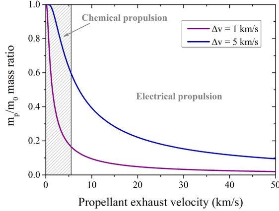
**Figure 1.** Ratio of the propellant mass to the initial mass as a function of the exhaust velocity  $v_e$  for two values of the velocity increment  $\Delta v$ . The dashed area corresponds to the domain of chemical propulsion with  $v_e$  below 5.5 km/s.
