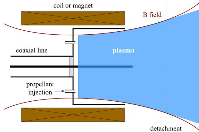
Figure 13. Schematic of the coaxial ECR plasma thruster [174].
