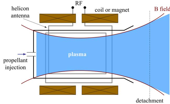
**Figure 12.** Schematic of a helicon plasma thruster.
