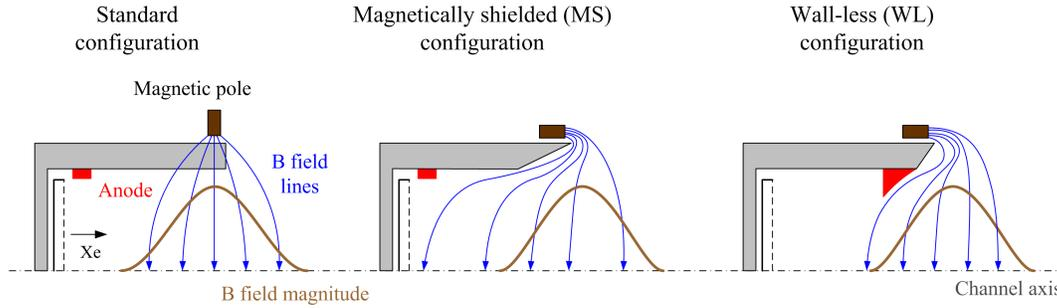
**Figure 9.** (Left) Basic configuration of a Hall thruster: the magnetic field lines intercept the walls. (Center) Magnetically shielded configuration: lines are parallel to the walls and they extend down to the anode. (Right) Wall-less configuration: the magnetic field lines are parallel to the anode that is placed at the exit plane.
