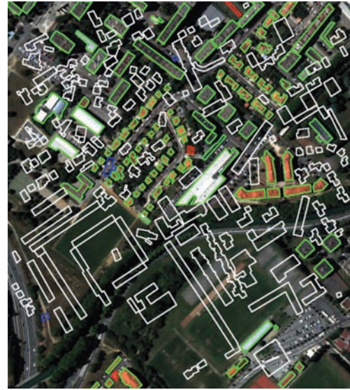
Fig. 7. Result of DB verification with the Toulouse data set for case 1, with the following colors: TP (in green), 108 buildings correctly accepted; FN (in red), three buildings wrongly rejected; FP (in blue), three objects wrongly accepted; and TN (in white), 145 objects correctly rejected.
