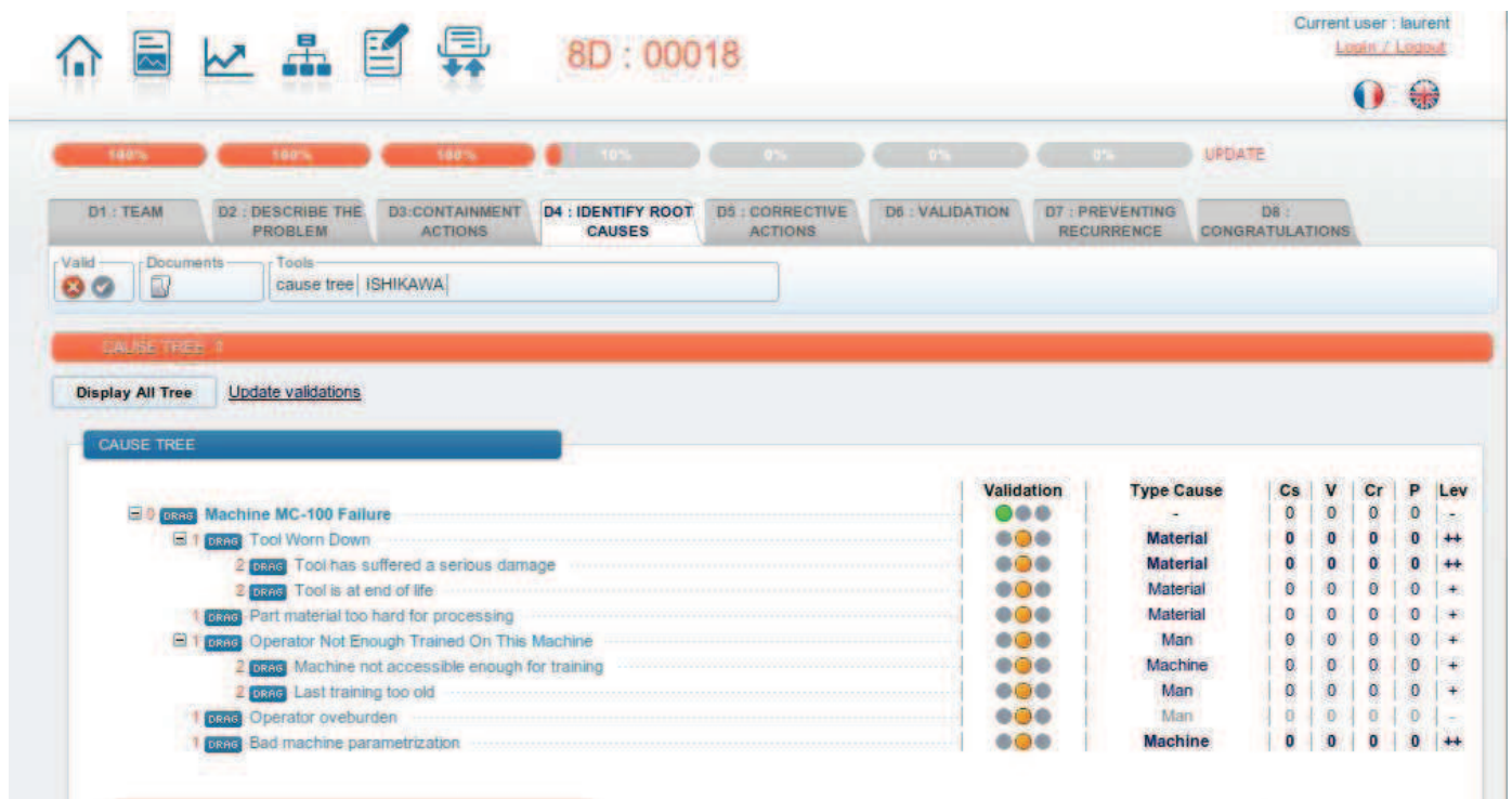
Figure 6. Root causes validation in the 8D method with T-REX
