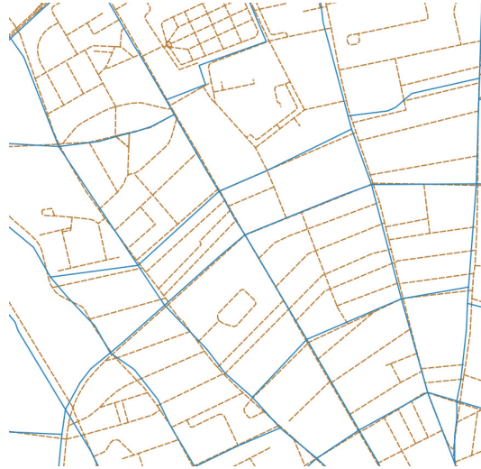
Figure 6: Two contemporary road networks (BDCarto from IGN in solid blue line and OpenStreetMap in brown dashed line) with a high difference of level of detail, which involves matching links of multiple cardinalities.
