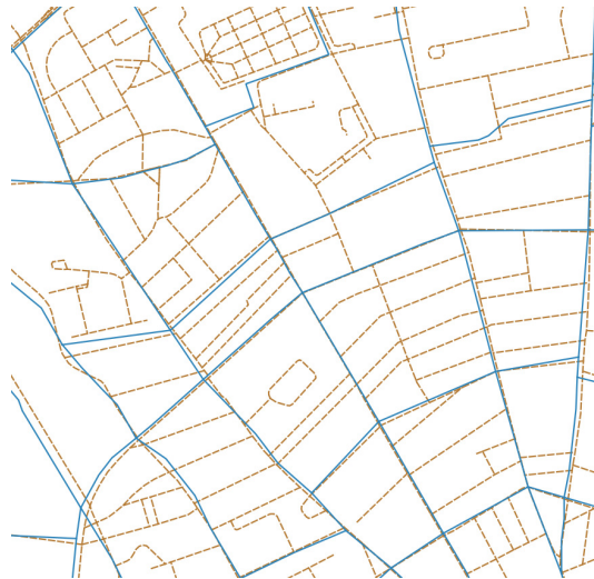
Figure 6: Two contemporary road networks (BDCarto from IGN in solid blue line and OpenStreetMap in brown dashed line) with a high difference of level of detail, which involves matching links of multiple cardinalities.
