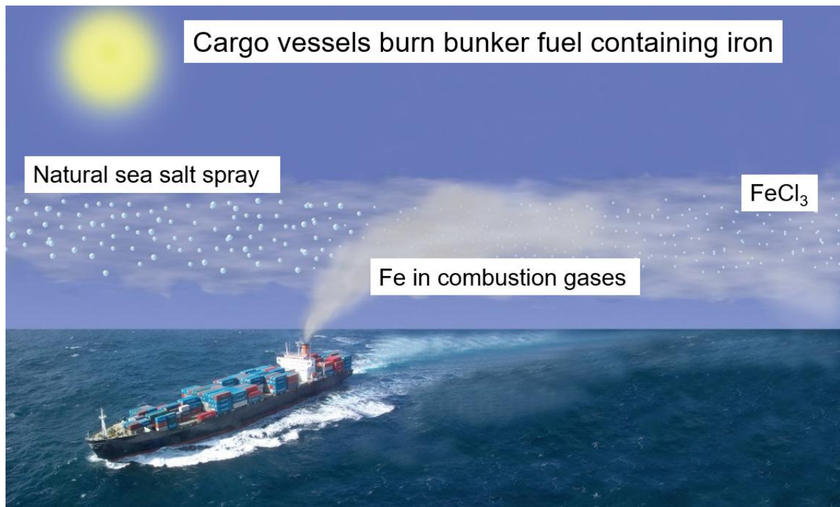
Figure 2: A container ship powered by bunker fuel mixed with commercially available iron additives [73, 74] which are sold to reduce black carbon and carbon monoxide (CO) emissions and to reduce fuel consumption. In the exhaust plume, the iron compounds react with sea salt to produce iron chloride ( \text{FeCl}_3 ), which under sunlight generates Cl atoms [69] that oxidize \text{CH}_4 16 times faster than ^{\circ}\text{OH} radicals [71].
