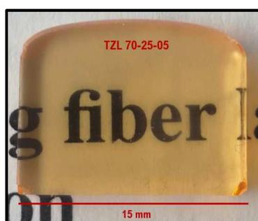
Fig. 5. Picture of TZL 70-25-05 bulk
