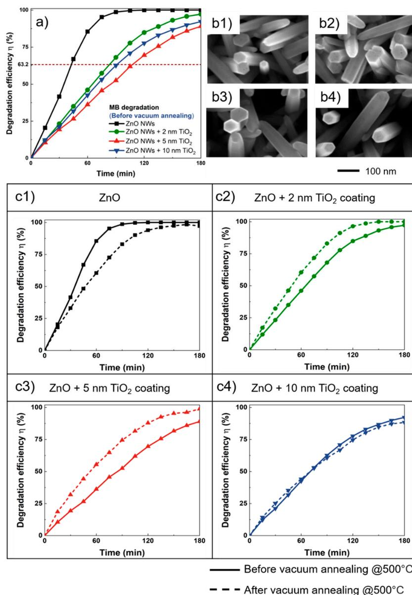
**Figure 4.** (a) Comparison of the photodegradation efficiency of MB among the different TiO<sub>2</sub> coating thicknesses from 0 to 10 nm. (b) The SEM photos of the ZnO NWs before (b1) and after vacuum-annealing (b2), 2 nm TiO<sub>2</sub>-coated ZnO NWs before (b3) and after vacuum-annealing (b4). (c1–c4) Comparison of photodegradation efficiency of different samples before and after vacuum-annealing.
