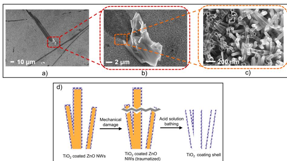
**Figure 3.** (a–c) Zoomed SEM views of 10 nm ALD TiO<sub>2</sub> coating on ZnO NWs after bathing in pH 3 aqueous solution for 30 min. (d) A schematic of the protective effect of the TiO<sub>2</sub> coating.
