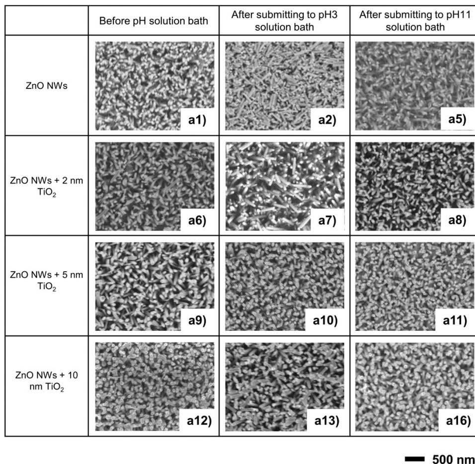
**Figure 2.** SEM images of the effect of TiO<sub>2</sub> coating thickness on ZnO NWs in strong acid/alkaline aqueous solutions.
