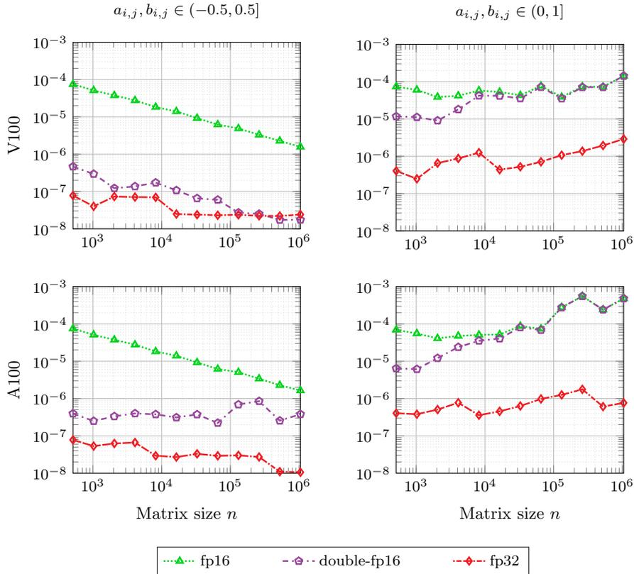
FIG. 4.2. Componentwise relative error of GPU implementations of algorithms for computing the product  $AB$ . The methods and arithmetics used are discussed in section 4.2.2. The double-fp16 matrices  $A \in \mathbb{R}^{16 \times n}$  and  $B \in \mathbb{R}^{n \times 16}$  have entries sampled uniformly at random from the interval at the top.
