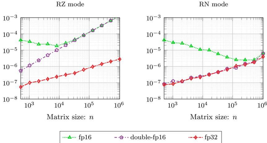
FIG. 4.3. Componentwise relative error of algorithms for computing the product  $AB$  using simulated block FMAs. The methods and arithmetics used are discussed in section 4.3. Two rounding modes are used: round-toward-zero (left) and round-to-nearest (right). The double-fp16 matrices  $A \in \mathbb{R}^{16 \times n}$  and  $B \in \mathbb{R}^{n \times 16}$  have entries sampled uniformly at random from the interval  $(0, 1]$ .
