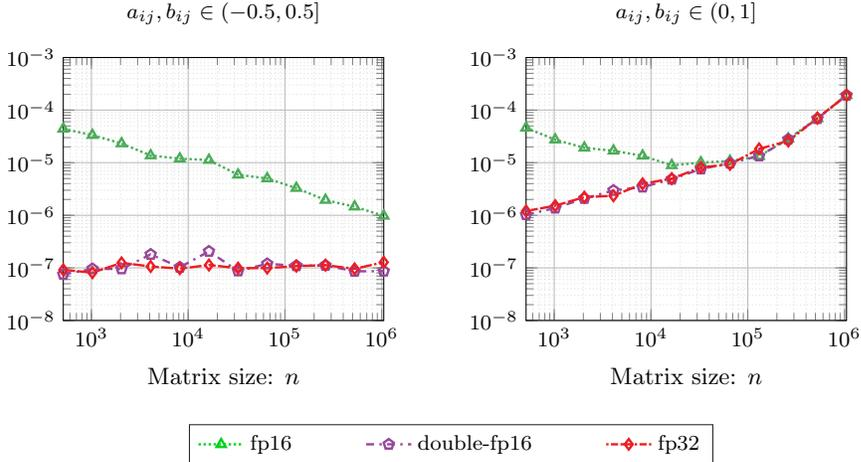
FIG. 3.1. Componentwise relative error of algorithms for computing the product  $AB$ . The methods and arithmetics used are discussed in section 3. The double-fp16 matrices  $A \in \mathbb{R}^{16 \times n}$  and  $B \in \mathbb{R}^{n \times 16}$  have entries sampled uniformly at random from the interval at the top.
