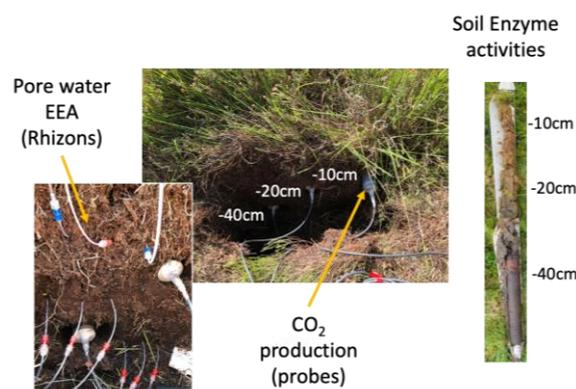
**Figure 2.** Depth profile installed in La Guette to monitoring EEA in pore water and CO<sub>2</sub> production. In parallel, soil EEA were also measured.
