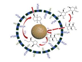
Scheme 9 Schematic illustration of the cascade reactions in a Ru-SO<sub>3</sub>H nanoreactor (Reproduced from Ref. 72)
