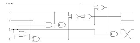
Figure B.3: A circuit implementation of LITTLUN-S4. The symbols  $\square$ ,  $\square$  and  $\square$  represent the AND, OR and XOR gates respectively.
