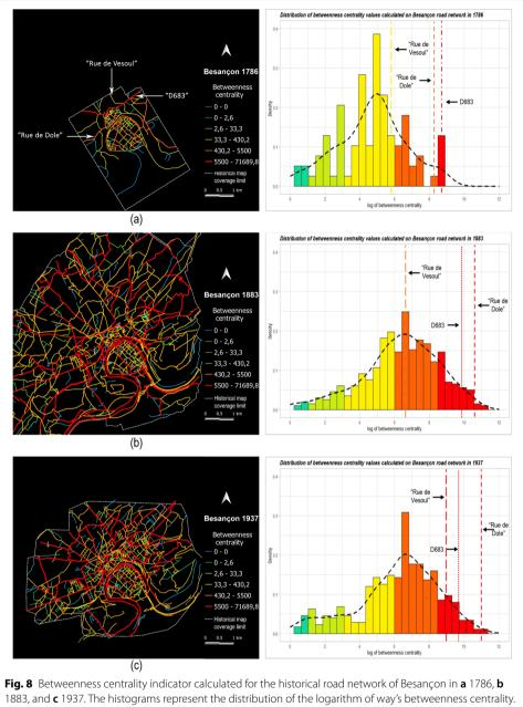
The dashed black line is the fitting of each histogram with a Gaussian mixture
