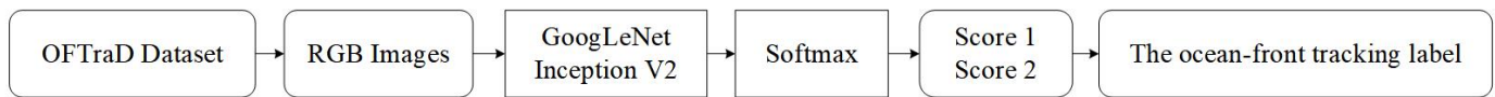
Figure 3. The procedure of the proposed ocean-front tracking algorithm. The input RGB images are fed to a GoogLeNet Inception network. Then, the softmax gives the probabilities of the input image belonging to the foreground or the background. The foreground images are used to track the ocean-front location in a video sequence.
