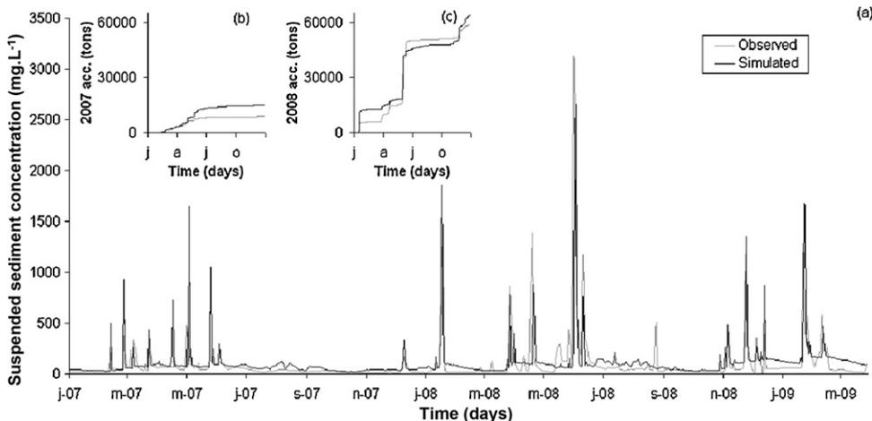
Fig. 4. Observed and simulated daily (a) suspended sediment concentration ( $\text{mg L}^{-1}$ ) at the Larra gauging station (January 2007–March 2009), (b) 2007 accumulation (tons) and (c) 2008 accumulation (tons).
