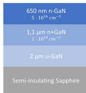
Figure 1. Schematic view of GaN epitaxy used in this study
