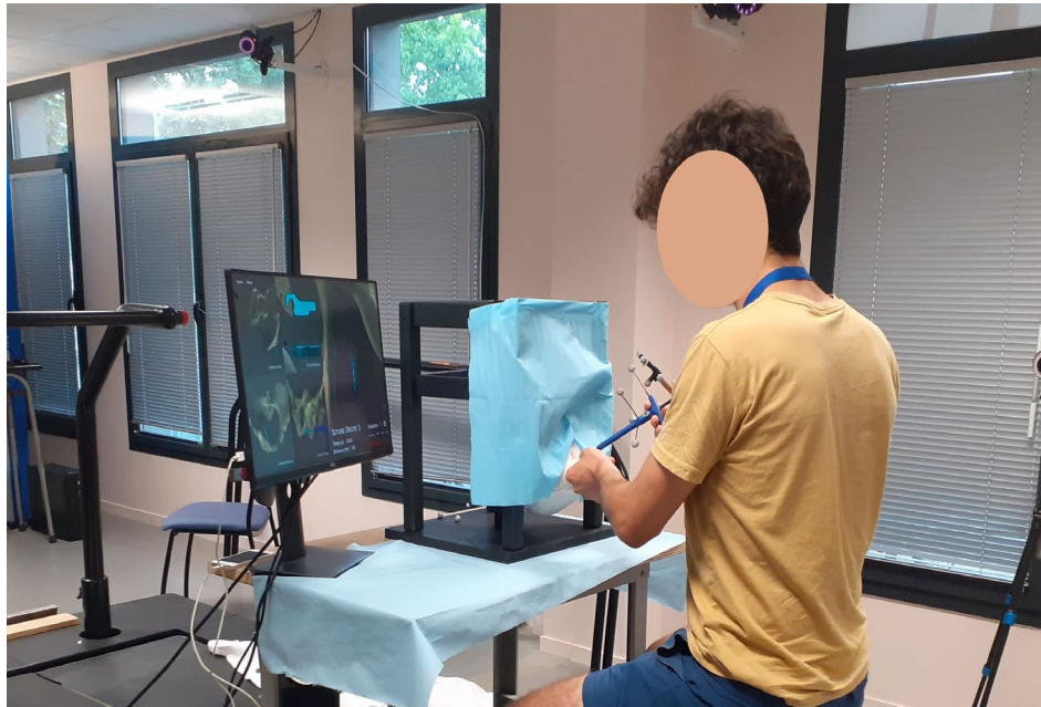
(a) The participant using the suturing device, while the pelvic mock-up is hidden by a curtain and the screen is displaying the information necessary for the participant to be guided to the target.
