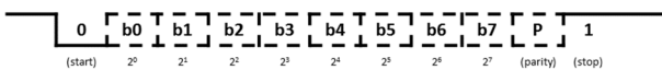
Fig. 3. UART character of PB DP: non-return-to-zero, 8 databits, 1 start and 1 stop bit, even parity.
