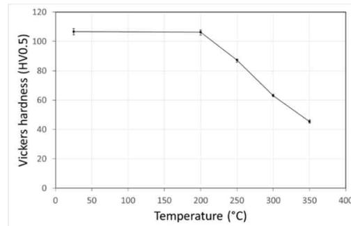
Figure 5: Material hardness as function of temperature. Bars represent the standard deviation.
