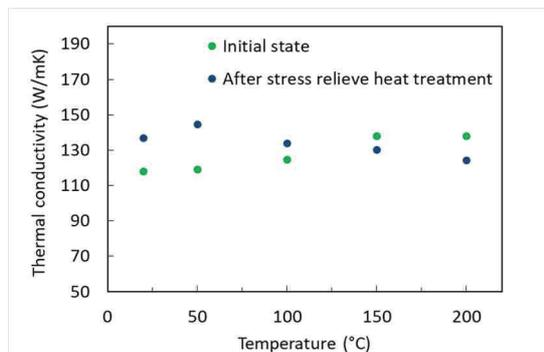
Figure 6: Thermal conductivity versus temperature at the initial state and after the stress relieve heat treatment.
