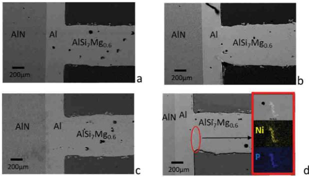
Figure 7: SEM images for the interfaces (a) Al at  $t_0$  (b) Al-Ni finish at  $t_0$ , (c) Al after thermal treatment and (d) Al-Ni finish after thermal treatment with focus region and EDX detection of precipitates.
