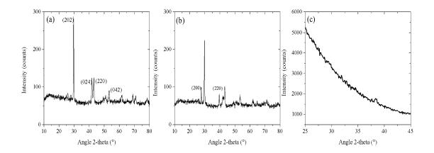
Fig. 2. Powder XRD patterns of  $Ge_9PbTe_{10}$  samples. Starting powder (a), SPS-prepared target (b), and GIXRD pattern obtained with the obtained thin film (c).
