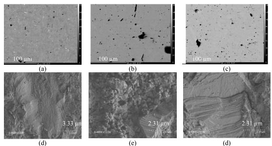
Fig. 1. Electron probe-microanalyser image of  $Ge_9PbTe_{10}$  (a),  $Ge_2TeSe$  (b) and  $Ge_4Te_3Se$  (c). SEM morphology of the fracture surface of  $Ge_9PbTe_{10}$  (d),  $Ge_2TeSe$  (e) and  $Ge_4Te_3Se$  (c) sintered targets.
