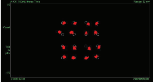
Fig. 2. Measured constellation diagram – 16QAM 2 Gbps at the test frequency 61 GHz.
