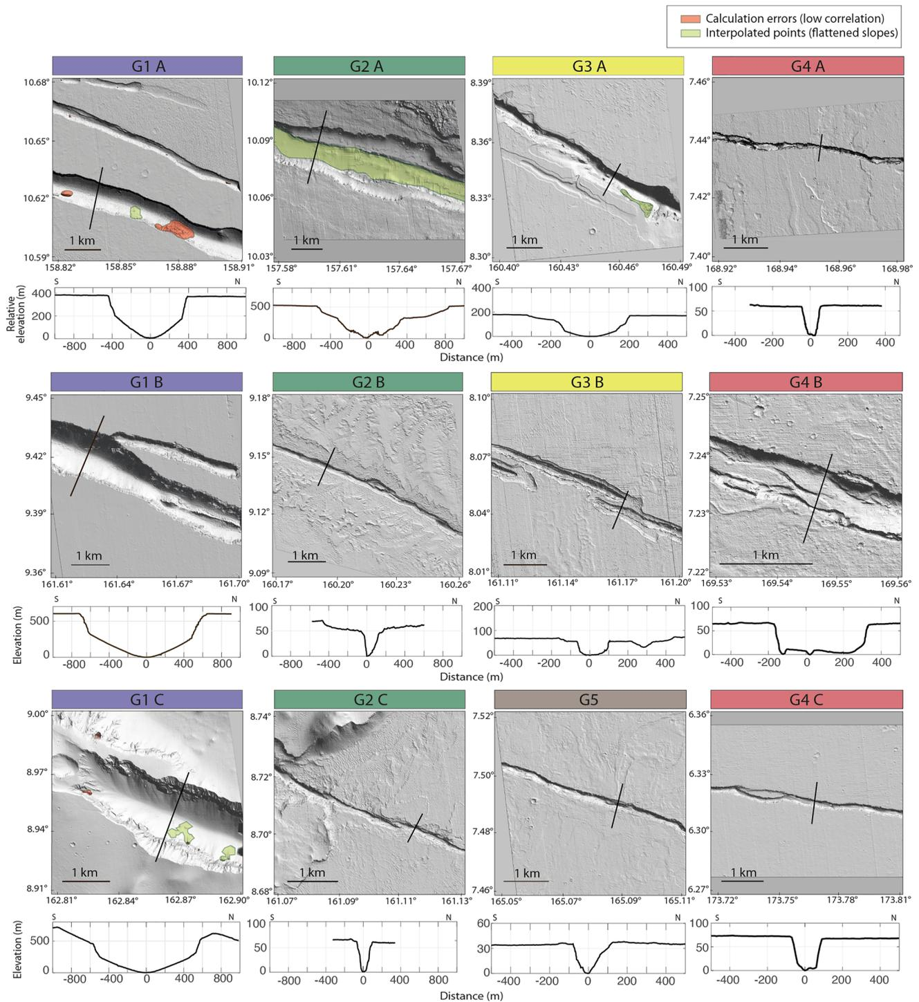
**Figure 5.** Digital Elevation Models (1 m/pixel) built from High-Resolution Imaging Science Experiment stereo pairs along the five main fossae (G1, G2, G3, G4, and G5) of Cerberus Fossae (see locations on Figure 1). One across strike relative topographic profile is shown below each DEM (see Figure S2 in Supporting Information S1 for all and mean profiles).
