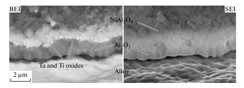
Fig. 3. SEM images of oxide film formed on surface of AM1 alloy.
