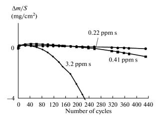
**Fig. 5.** Curves of cyclic oxidation of the AM1 alloy with different sulfur contents.
