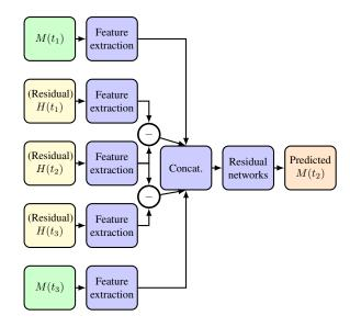
**Fig. 3**. Structure of the fusion block of CSTF.
