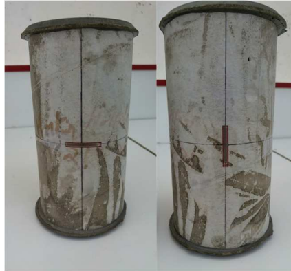
Figure 6: Prepared specimens with strain gauges
