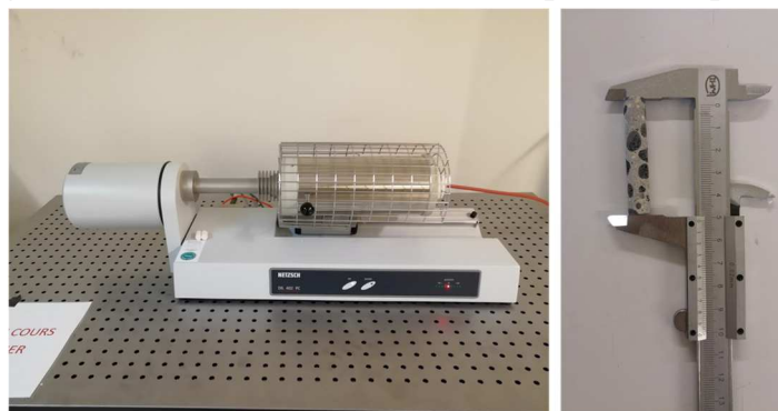
Figure 7: Dil 402-PC device and an example of a sample used
