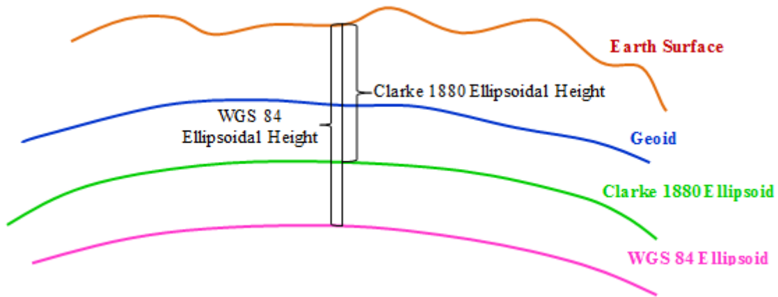
Fig. 1. Relationship between WGS84 and Clarke 1880 ellipsoids
