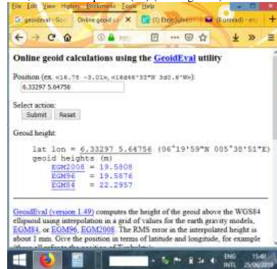
Figure 6: Processing of the GNSS Data Using Compass Software Figure 7: Computation of the Global Geoid Heights of the Points Using GeoidEval Software
