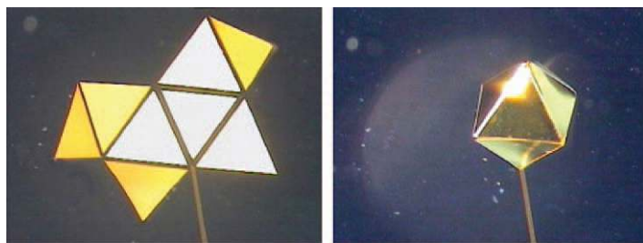
Figure 12.9 Octahedron of PPy/Au bilayer hinge microactuators with rigid elements by M. Krogh et al. , Micromuscle AB, inspired by Smela et al. 82 Reproduced from ref. 122 with permission from Elsevier, Copyright 2007.
