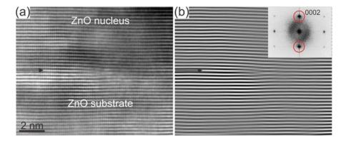
**Fig. 5** (a) High-resolution TEM image of the interface region between the ZnO nucleus and the Zn-polar ZnO single crystal. The arrow denotes the interface. (b) Corresponding 0002 Bragg image of the interface area through the use of a mask on the 0002 spatial frequencies to reveal only the (0002) planes. The inset shows the electron diffraction pattern with the 0002 peaks circled.
