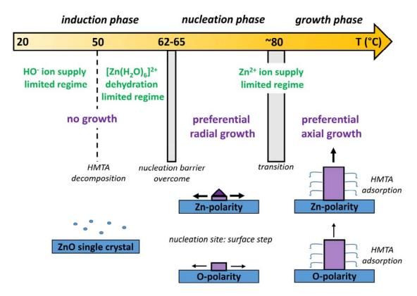
**Fig. 8** Schematic diagram describing the dominant physicochemical processes during the three phases of the formation of O- and Zn-polar ZnO NWs by CBD on O- and Zn-polar ZnO single crystals, respectively.
