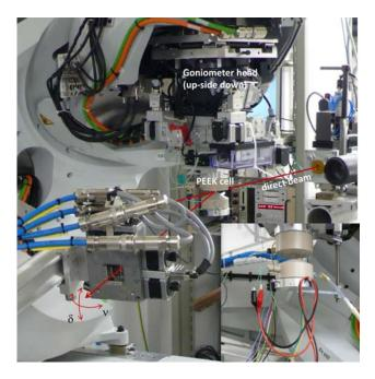
**Fig. 1** Picture of the X-ray transparent growth cell mounted on the  $\kappa$ -head of the goniometer of D2AM-BM02 beamline at ESRF at  $\chi = -90^{\circ}$ . The substrate surface was placed upside-down with the scattering vector pointed down to the floor. The inset presents a magnification of the growth cell composed of lower and upper reservoirs with the same volume, linked to the X-ray transparent cylindrical tube in which the sample sits.
