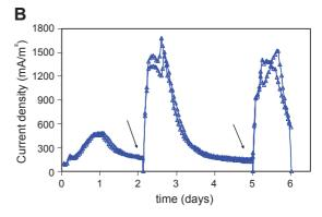
**Fig. 4.** Chronoamperometry at +0.1 V/SCE of graphite felt in compost leachate. A) Low- and extended-anodised, and B) extended-anodised electrodes with adsorbed dairy waste. Arrows indicate dairy waste addition; two similar experiments were performed simultaneously for each case.
