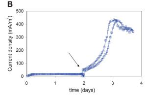
**Fig. 1.** Chronoamperometry at +0.1 V/SCE with compost leachate as inoculum and dairy waste as fuel. Arrow indicates A) replacement of the inoculum medium by dairy waste, and B) dairy waste addition into the inoculum medium.
