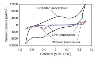
Fig. 2. Cyclic voltammetry  $(1\,\mathrm{mV/s})$  with graphite felt electrodes after low- or extended-anodisation in phosphate buffer.
