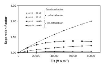
**Fig. 7.** Estimated separation factor versus the product of the electric field by the residence time  $(E \cdot \tau)$ . Operating conditions: mixture:  $\alpha$ -L,  $C_0 = 0.1 \, \mathrm{g \, L^{-1}}$  and  $\beta$ -L,  $C_0 = 0.2 \, \mathrm{g \, L^{-1}}$ ; separation configuration.
