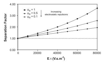
**Fig. 2.** Variation of the calculated separation factor versus the product of the electric field by the residence time  $(E \cdot \tau)$ : influence of electrostatic interactions. Case 1: target protein A;  $u_{miA} \times u_{miB} < 0$ ;  $|u_{miA}| = |u_{miB}| = 10^{-8} \text{ V m}^2 \text{ s}^{-1}$ ;  $\phi_A = 1$ ;  $u_{eo} = 2 \times 10^{-9} \text{ V m}^2 \text{ s}^{-1}$ ; membrane and protein B: same sign of charge; separation configuration.
