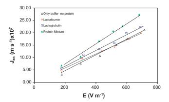
**Fig. 4.** Variation of the electro-osmotic flux versus the electric field. Operating conditions: buffer: Mes-histidine at pH 6,  $Q = 100 \text{ mL h}^{-1}$ , membrane MWCO 30 kDa.
