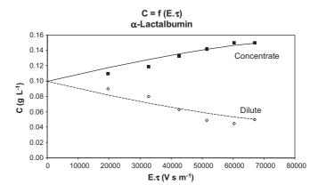
**Fig. 5.** Comparison between experimental (points) and calculated (curves) outlet concentrations versus the product of the electric field by the residence time ( $E \cdot \tau$ ). Operating conditions: single solution of  $\alpha$ -L,  $C_0$  = 0.1 g L<sup>-1</sup>; Tris-Mes buffer at pH 8; membrane MWCO 30 kDa; separation configuration.
