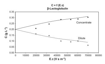
**Fig. 6.** Comparison between experimental (points) and calculated (curves) outlet concentrations versus the product of the electric field by the residence time ( $E \cdot \tau$ ). Operating conditions: single solution of  $\beta$ -L,  $C_0$  = 0.2 g L<sup>-1</sup>; Tris-Mes buffer at pH 8; membrane MWCO 30 kDa; separation configuration.
